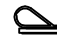
PEMKO HSS2000x88 CATEGORY 'G' EDGE SEALING SYSTEM (USED ON FIRE RATED PRODUCTS)
